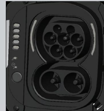
The new 500e is equipped with a CCS\* COMBO 2 Smart Charging Port that enables both public AC and DC charging as well as simple domestic AC charging. The port is positioned in the right rear side of the vehicle and gives immediate feedback on the charging status as well as possibility to manage set charging schedule or immediate charging.
